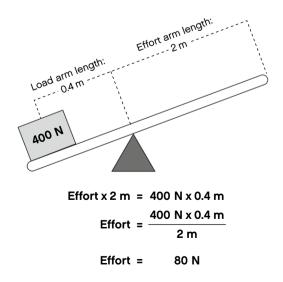
Using this 1st class lever to lift a 400 N load would only need an effort of 80 N. However, the effort end of the lever must move five times the distance of the load.
