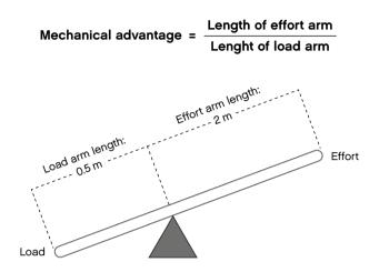
The mechanical advantage of this 1st class lever is:
